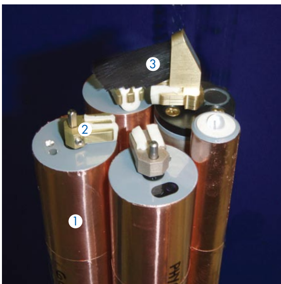
Anti-fouling kits include 1) copper tape, 2) wiper assemblies with larger pads, 3) extended brushes, and 4) sonde guard
